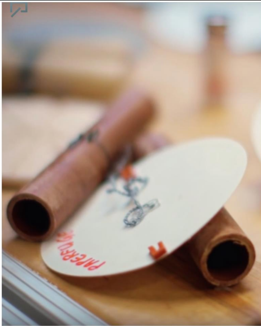
Paperfuge A 20-cent hand-powered centrifuge
